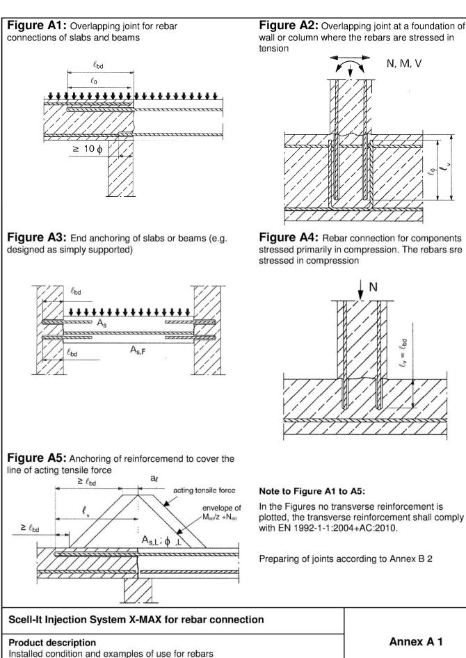
Figure A2: Overlapping joint at a foundation of a wall or column where the rebars are stressed in tension
