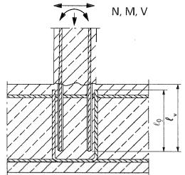
Figure A4: Rebar connection for components stressed primarily in compression. The rebars sre stressed in compression
