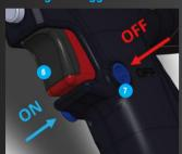
Lock the trigger 6 when the tool is not in use. To lock the trigger, push trigger lock 7 at OFF site, the tool will not operate.
