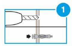
Drill the support to the specified diameter.
