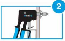
Insert the pliers between the head of the screw and the collar of the dowel.
