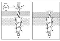
Insert the screw in the center of the plug and then, tight through the fixing piece
