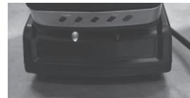
Red light on the charger: the battery has to be charged
