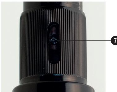
3. Insert the pin (8) into the hole (7) in order to block the mandrel rotation.
