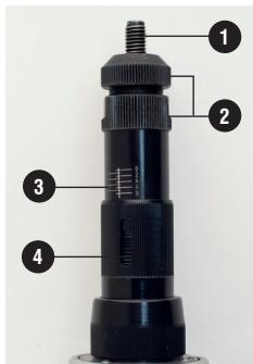
According to the nut and the support thickness the stroke must be adjusted to provide ideal installation.
