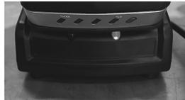
Red light on the charger: the battery has to be charged
