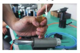
5. Test the tool stroke, if the stroke still getting less, it means there could be air in the oil cyliner, then the extra air needs to be released from the tool:
