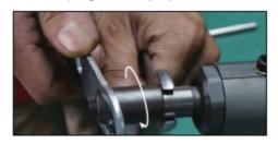
4. Install the front sleeve (#2) and nosepiece (#1):
