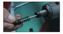
2. Put 3-jaw set (#4) into clamping sleeve
