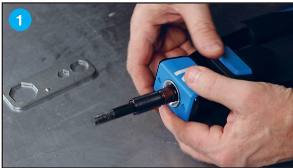
Fit the mandrel and nose that corresponds to the diameter of the rivnut (M4, M5, M6, M8 or M10).
