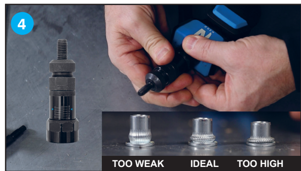
To adjust the stroke: loosen the retaining nut then turn the anvil and sleeve parts to increase/reduce the stroke (possible adjustment from 1 to 10mm). Then retighten. Diagram shows the ideal rivnut deformation.
