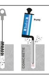
2. Clean the hole Remove dust and debris from the hole with a pump and/or a suitably sized brush (preferably a wire brush).
