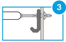
Remove the screw to position the object to be fixed.
