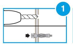
Drill the support to the specified diameter. Insert the dowel flush with the hole. Unscrew the screw by +/-4 mm.
