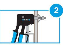
Insert the pliers between the head of the screw and the collar of the dowel.
